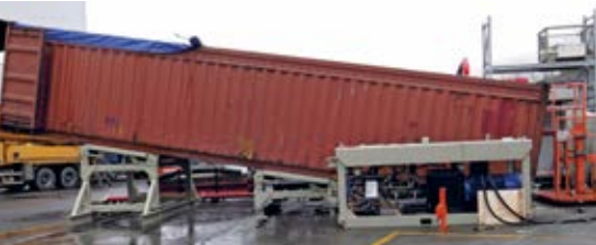
The conditions at the planned operational site were simulated in the container positioned at a 10 ° slant.
