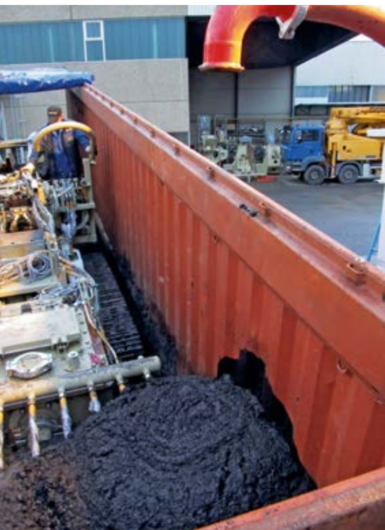
The KOS 1060 DSC runs into the coal-fly ash mixture.
